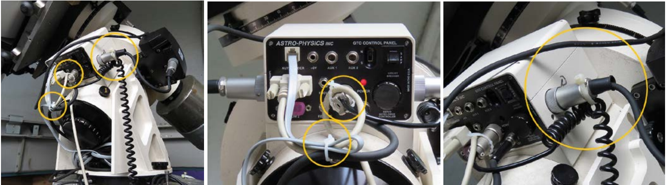
Picture center: Detail view of the merged cable RS 232, Guiding and Soannungsversorgung mount and strain relief connector on the manual control unit.
