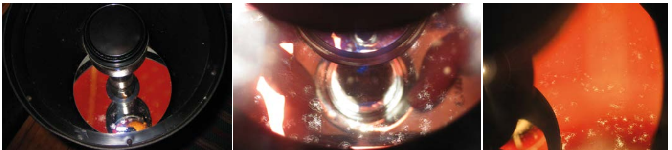
These images show the view into a Schmidt-Cassegrain, which was stored at moist-warm climate near the ocean for some years. Even the closed tube of a SC was no protection against fungus under this conditions.
