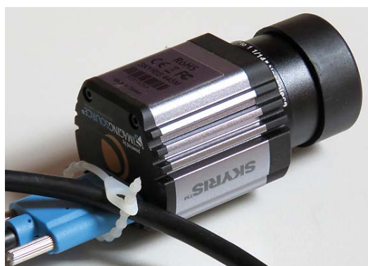
Figure 01: Re-open cable tie (knot ribbon). Figure 02 and 03: Cable loop directly to the USB 3.0 connector of SkyRis camera with tape knot to secure
