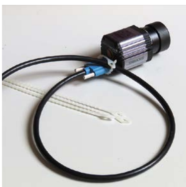
Figure 01: Re-open cable tie (knot ribbon). Figure 02 and 03: Cable loop directly to the USB 3.0 connector of SkyRis camera with tape knot to secure
